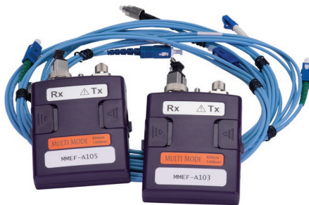
Multimode (encircled flux) modules
